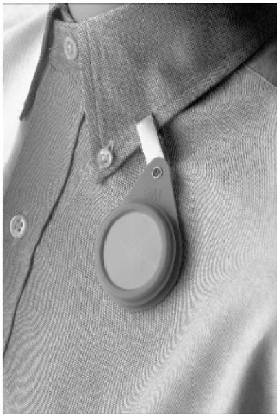
Figure 1.3. Passive dosimeter collects gases and vapors without a sampling pump. (Courtesy of SKC, Inc.)
